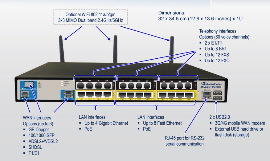
Note: The figure above is used only as an example. The number and type of port interfaces depends on the ordered model.
